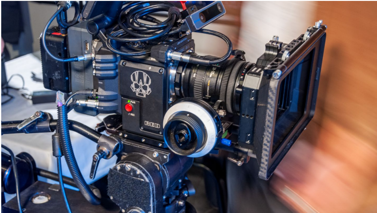
The mechanical focus knob with a ring on it for marking specific distances. In this configuration the focus puller would have to be alongside the camera to change focus.
