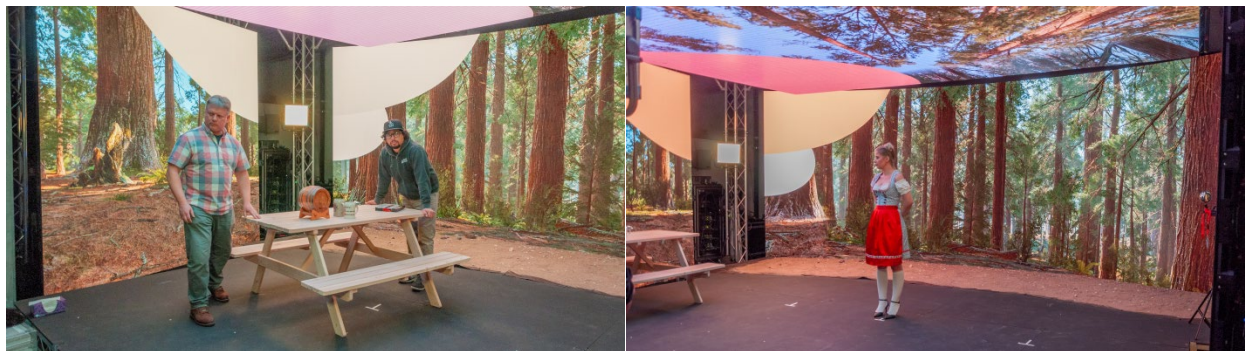
Large sections of the LED displays that weren't seen by the camera were used to light the set
