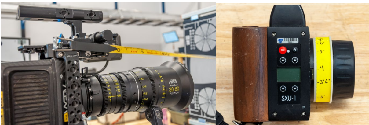
A tape measure is attached to the camera at the plane of the sensor, clearly marked on the camera and the remote control belonging to this particular focus system.
