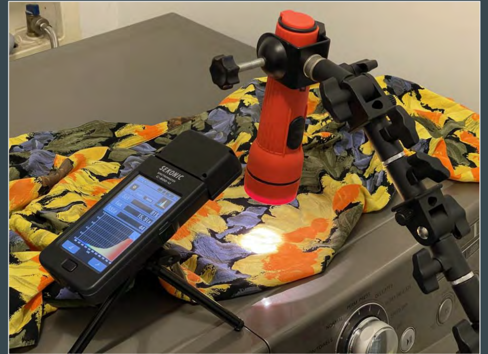
Laundry room reflectometry with a Sekonic C-800 Spectral Light Meter
